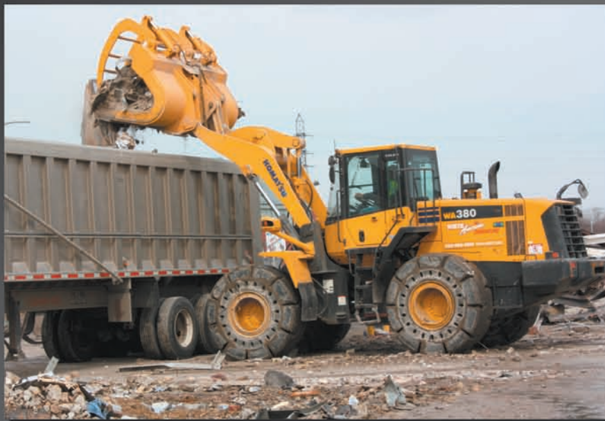
Loading debris with a 380 Komatsu front-end loader.
